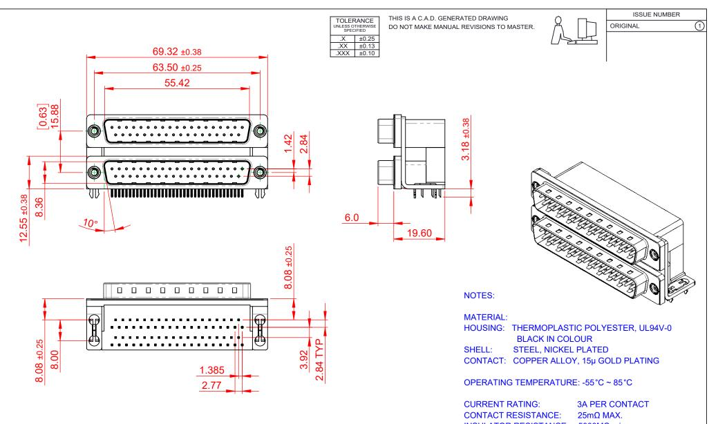
INSULATOR RESISTANCE: 5000MΩ min. DIELECTRIC WITHSTANDING VOLTAGE: 1000V AC rms
