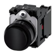
Pushbutton, 22 mm, round, plastic, black, pushbutton, raised, momentary contact type, with holder 1 NC, screw terminal, with laser labeling, symbol number according to, ISO 7000 or IEC 60417
