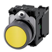
Pushbutton, 22 mm, round, plastic with metal front ring, yellow, pushbutton, flat, momentary contact type, with holder, 1 NO, screw terminal, with laser labeling, inscription or symbol Customer-specific selection with SIRIUS ACT configurator (CIN)
