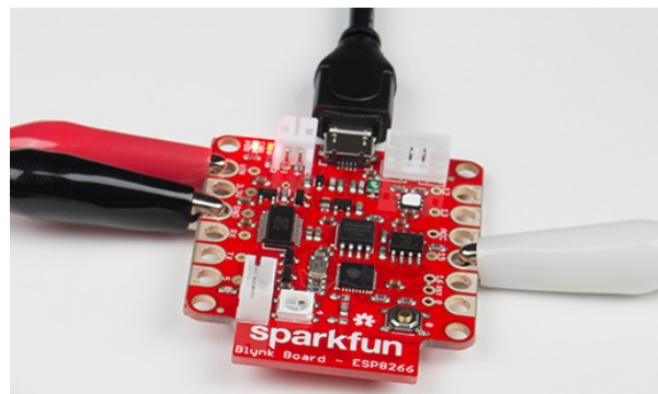
Alligator clips clipped onto the Blynk Board, interfacing it with the physical world.
