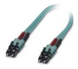
Assembled FO cable, zip cord cable, multi-mode fiberglass 50/125  $\mu$ m, OM3, plug: LC/LC, degree of protection: IP20, for installation in cable ducts or control cabinets, length: 1 m
