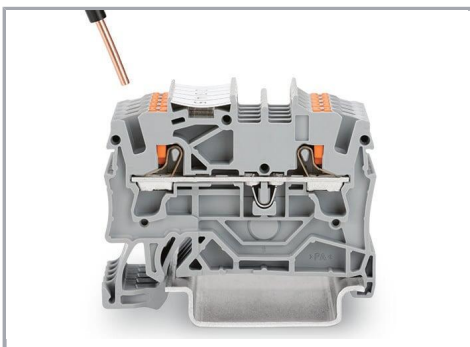
Push-in termination of solid and ferruled conductors
