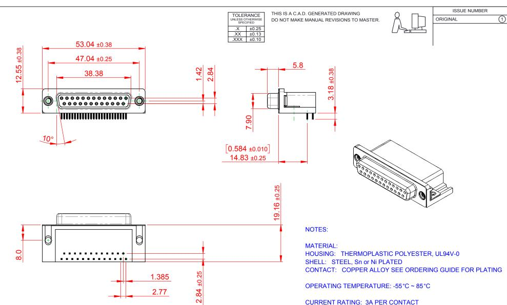
CONTACT RESISTANCE: 25mΩ MAX. INSULATOR RESISTANCE:  $5000M\Omega$  min. **DIELECTRIC**
