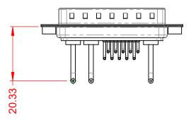
10A (CURRENT) POWER/CO-AX CONTACT RATING: (IF PRESENT) SIGNAL CONTACT CURRENT RATING: 5A PER CONTACT SIGNAL CONTACT RESISTANCE:  $10m\Omega$  MAX. INSULATOR RESISTANCE:
