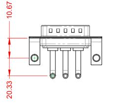
POWER/CO-AX CONTACT RATING: (IF PRESENT) SIGNAL CONTACT CURRENT RATING: 5A PER CONTACT SIGNAL CONTACT RESISTANCE:  $10m\Omega$  MAX.
