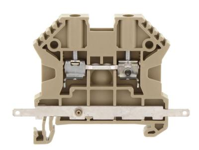
Feed-through terminal, Screw connection, Mounting type: Mounting rail TS 35/7.5, Rated cross-section: 2.5 mm², Width: 5 mm, Colour: Red
