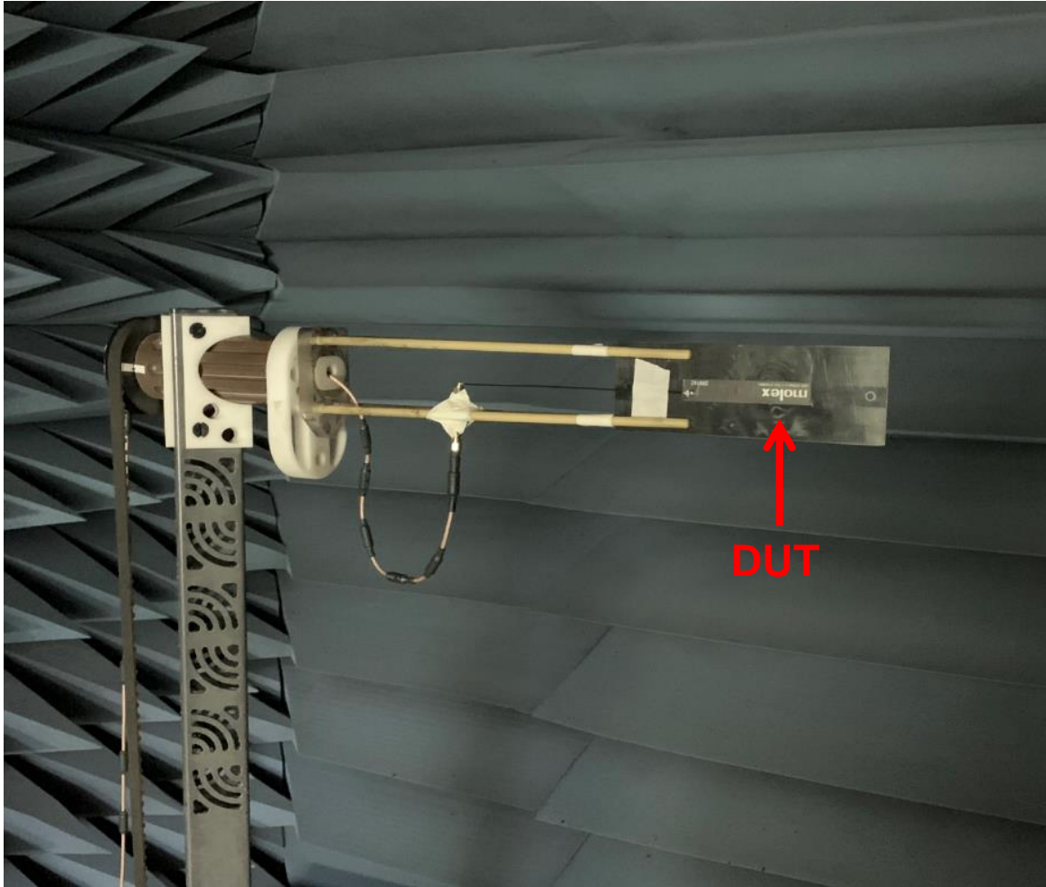
FIGURE4.1.3 ANTENNA LOADED WITH PC/ABS BLOCK OF 1.5MM THICKNESS TESTED IN OTA CHAMBER
