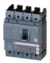
circuit breaker 3VA5 UL frame 250 breaking capacity class C 100kA @ 480V 4-pole, line protection TM210, FTFM, In=125A overload protection Ir=125A fixed short-circuit protection Ii=10 x In N conductor protection 100% without connection
