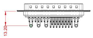
20A (CURRENT) POWER/CO-AX CONTACT RATING: (IF PRESENT) SIGNAL CONTACT CURRENT RATING: 5A PER CONTACT SIGNAL CONTACT RESISTANCE:  $10m\Omega$  MAX. INSULATOR RESISTANCE: 5000MΩ min.
