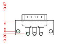
40A (CURRENT) POWER/CO-AX CONTACT RATING: (IF PRESENT) SIGNAL CONTACT CURRENT RATING: 5A PER CONTACT SIGNAL CONTACT RESISTANCE:  $10m\Omega$  MAX.
