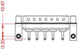
10A (CURRENT) POWER/CO-AX CONTACT RATING: (IF PRESENT) SIGNAL CONTACT CURRENT RATING: 5A PER CONTACT SIGNAL CONTACT RESISTANCE:  $10m\Omega$  MAX.
