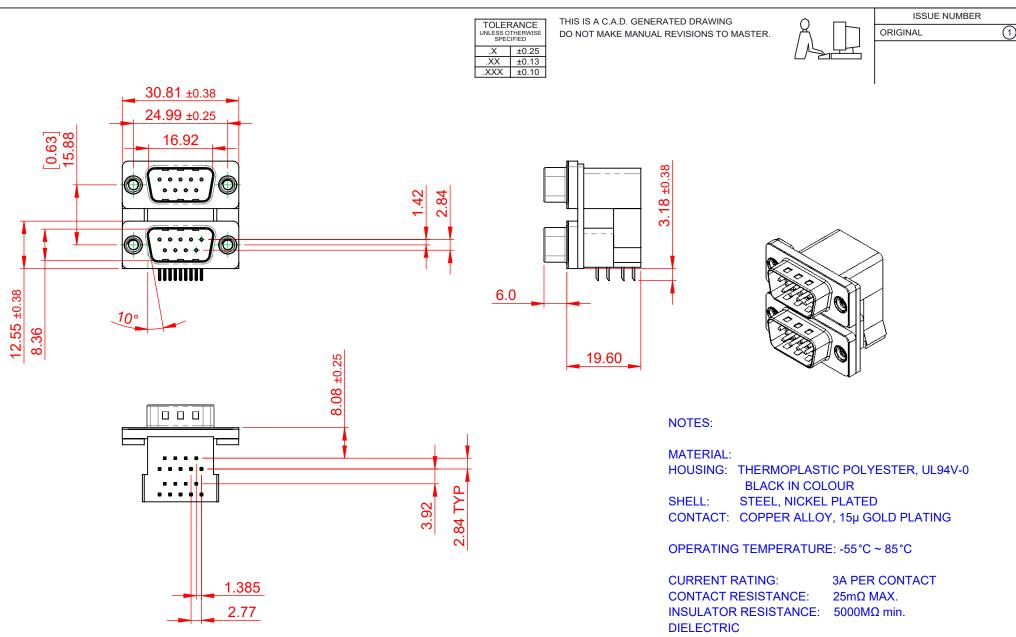
WITHSTANDING VOLTAGE: 1000V AC rms
