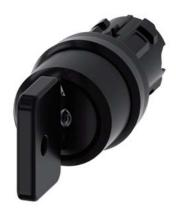
Key-operated switch O.M.R, 22 mm, round, plastic, lock number 73034, black, with 2 keys, 3 switch positions I-O-II, latching, actuating angle 2x45°, 10:30h/12h/13:30h, key removal O, with laser labeling, upper case
