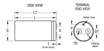
General Information Series ALS30 Dielectric Aluminum Electrolytic Description Screw Terminal, Aluminum Electrolytic RoHS Yes AEC-Q200 No Component 690 g Weight Dimensions D And L Include Sleeving. MS (MxH) = Notes M12x16. Mounting Clamp (Sold Separately): V11 Shelf Life 156 Weeks
