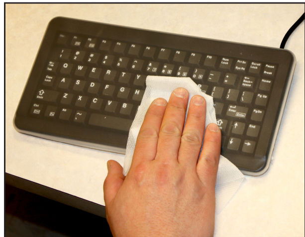
Traditional keyboards, and even some sealed, anti-microbial keyboards, have areas that are difficult to clean. Conversely, keyboard covers with a thin smooth surface provide protection from debris and make it simple to clean the entire surface.
