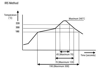
Note: Temperature profile shows printed circuit board surface temperature on the relay terminal portion. Please consult KEMET if you wish to use a temperature profile other than above.
