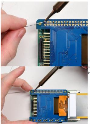
Heat up your soldering iron, and grab some solder. Start by tack-soldering one of the corners. Then you can re-heat that solder point and adjust the circuit board to make it sit flat.
