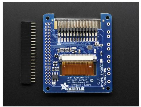
Check also on the back that the TFT is attached and that the flex connector is seated into the onboard FPC socket.
