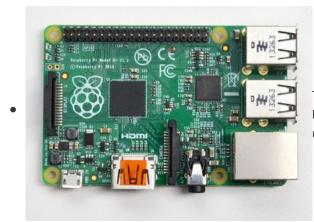
The easiest way to attach the header is if you have a Raspberry Pi as a 'stand' - make sure its powered off & unplugged!
