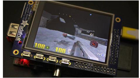
The Ideal: Adafruit's PiTFT displays are razor sharp. Whereas small composite screens on the Raspberry Pi usually require some video scaling (resulting in blurriness), PiTFT uses the GPIO header, digitally controlled pixel-by-pixel for a rock steady image. Though not a *lot* of pixels, it works great for retro gaming (and the display neatly stacks above the board, no side protuberances for video cables).
