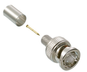
307-HP-102 BNC Male 3PC Crimp-Crimp, 75 Ohm, 1-4GHz
