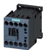
Power contactor, AC-3 16 A, 7.5 kW / 400 V 1 NO, 380 V AC, 50/60 Hz 3-pole, Size S00 screw terminals
