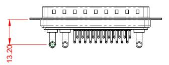
30A (CURRENT) POWER/CO-AX CONTACT RATING: (IF PRESENT) SIGNAL CONTACT CURRENT RATING: 5A PER CONTACT SIGNAL CONTACT RESISTANCE:  $10m\Omega$  MAX. **INSULATOR RESISTANCE:** 5000MΩ min.
