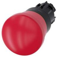
EMERGENCY STOP mushroom pushbutton, 22 mm, round, plastic, red, 40 mm, positive latching, acc. to EN ISO 13850, pull-to-unlatch mechanism, with laser labeling, upper case and lower case, always upper case at the beginning of the word
