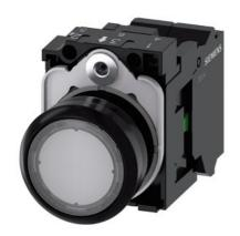
Illuminated pushbutton, 22 mm, round, plastic, clear, pushbutton, flat, momentary contact type, with holder, 1NO, LED module with integrated LED 24 V AC/DC, spring-type terminal, with laser labeling, upper case
