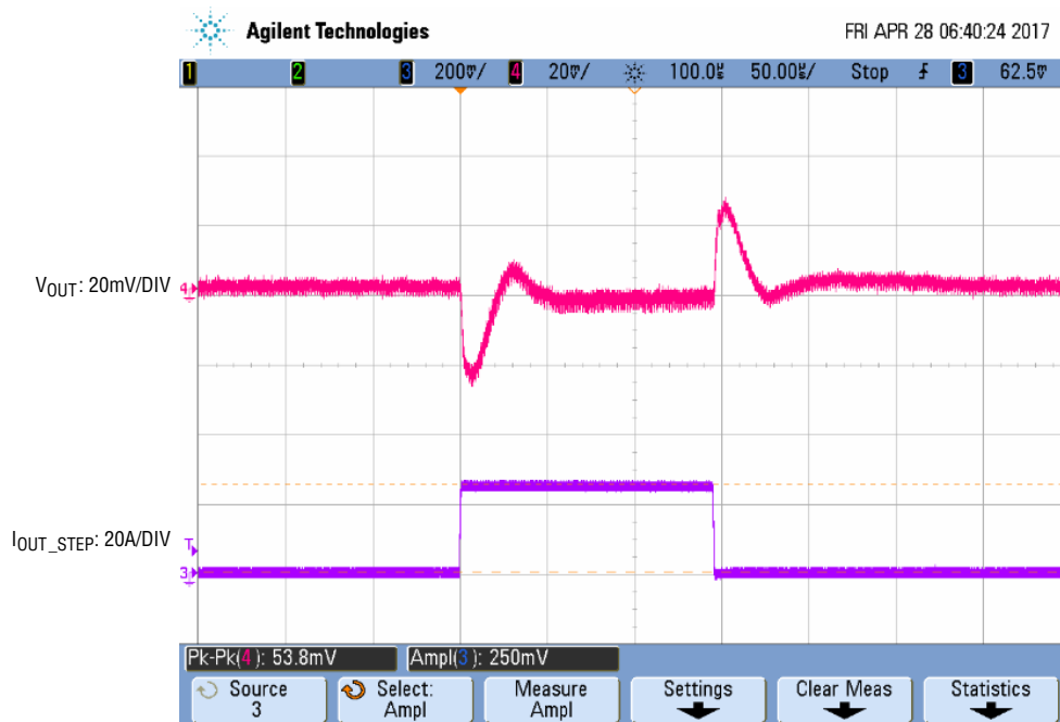
Figure 3. Measured Load Transient V IN = 12V, V OUT = 1.0V, I STEP = 0A to 25A
