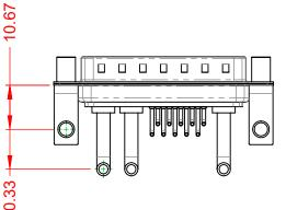
30A (CURRENT) POWER/CO-AX CONTACT RATING: (IF PRESENT) SIGNAL CONTACT CURRENT RATING: 5A PER CONTACT SIGNAL CONTACT RESISTANCE:  $10m\Omega$  MAX. **INSULATOR RESISTANCE:**
