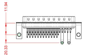
POWER/CO-AX CONTACT RATING:20A (CURRENT)(IF PRESENT)SIGNAL CONTACT CURRENT RATING:5A PER CONTACTSIGNAL CONTACT RESISTANCE:10mΩ MAX.INSULATOR RESISTANCE:5000MΩ min.
