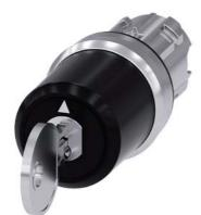
key-operated switch Siemens, 22 mm, round, metal, shiny, lock number SSG10, with 2 keys, 3 switch positions I>O<II, momentary contact on the left, latching on the right, actuating angle 2x45°, 10:30h/12h/13:30h, key removal O+II, with laser labeling, inscription or symbol customer-specific selection with SIRIUS ACT configurator (CIN)
