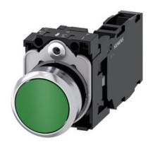
Pushbutton, 22 mm, round, metal, shiny, green, pushbutton, flat, momentary contact type, 1 NO+1 NC, screw terminal, with laser labeling, upper case and lower case, always upper case at the beginning of the word
