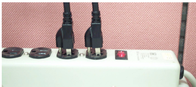
Figure 3.10: Power cord plugs should have same orientation in the socket/ 插座上电源线方向相同 / 插座上的電源線方向應相同
