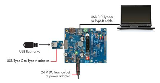
Note that any USB device can be used instead of a flash drive with the setup shown in step 3.
