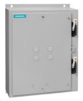
Duplex starter w/o alternator, Size 1 3/4, Three phase full voltage, Solidstate overload relay, OLR amp range 10-40A, 208VAC 60Hz coil, Combination type, Two 40A circuit breakers, Enclosure NEMA type 12, Dust/drip proof for indoors
