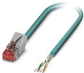
Assembled Ethernet cable, CAT5e, shielded, 2-pair, 26 AWG stranded (7-wire), RAL 5021 (water blue), RJ45 plug/IP20 to free cable end, line, length: 0.5 m
