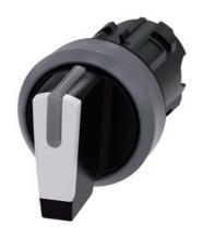
Selector switch, illuminable, 22 mm, round, plastic with metal front ring, white, selector switch, short, 3 switch positions I-O-II, latching, actuating angle  $2x45^{\circ}$ , 10:30h/12h/13:30h, with laser labeling, upper case and lower case, always upper case at beginning of line
