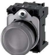
Indicator lights, 22 mm, round, plastic, clear, lens, smooth, with holder, LED module with integrated LED 110 V AC, screw terminal, with laser labeling, upper case and lower case, always upper case at the beginning of the word
