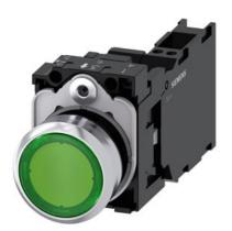
Illuminated pushbutton, 22 mm, round, metal, shiny, green, pushbutton, flat, momentary contact type, with holder, 1 NO+1 NC, LED module with integrated LED 24 V AC/DC, spring-type terminal, with laser labeling, lower case
