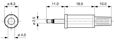
Cable diameter max. 4.0 mm
