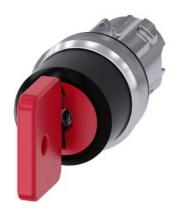
Key-operated switch O.M.R, 22 mm, round, metal, shiny, lock number 73037, red, with 2 keys, 3 switch positions I-O-II, latching, actuating angle 2x45°, 10:30h/12h/13:30h, Key removal I+O+II, with laser labeling, upper case and lower case, always upper case at the beginning of the word
