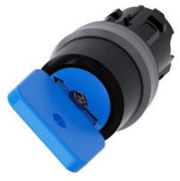
Key-operated switch O.M.R, 22 mm, round, plastic with metal front ring, lock number 73038, blue, with 2 keys, 2 switch positions O<I, momentary contact type, Actuating angle 45°, 10:30h/12h, key removal O, with laser labeling, upper case and lower case, always upper case at the beginning of the word
