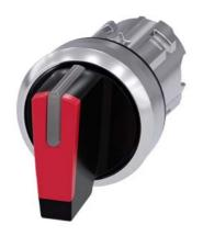
Selector switch, illuminable, 22 mm, round, metal, shiny, red, selector switch, short, 3 switch positions I-O-II, latching, actuating angle 2x45°,  $10:30h/12h/13:30h,\,Z=50$ -unit packaging
