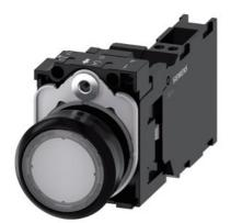
Illuminated pushbutton, 22 mm, round, plastic, clear, pushbutton, flat, momentary contact type, with holder, 1 NO+1 NC, LED module with integrated LED 110 V AC, spring-type terminal, with laser labeling, upper case
