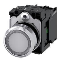
Illuminated pushbutton, 22 mm, round, Metal, shiny, transparent, pushbutton, flat, momentary contact type, with holder, 1NO, LED module with integrated LED 230 V AC, screw terminal, with laser labeling, lower case
