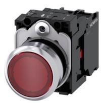
Illuminated pushbutton, 22 mm, round, metal, shiny, red, pushbutton, flat, momentary contact type, with holder, 1NC, LED module with integrated LED 230 V AC, screw terminal, with laser labeling, lower case
