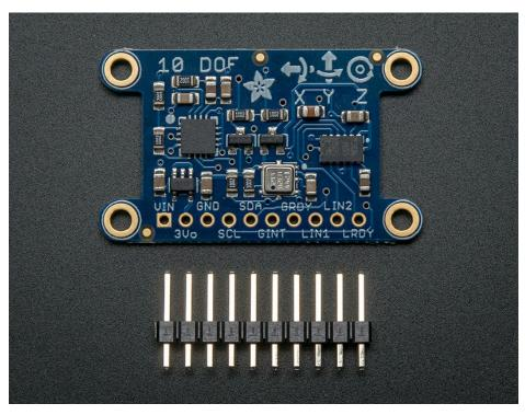
Please note that there is a small cosmetic error on the first revision of these boards (shown above). The straight X arrow for the accelerometer should be pointing in the opposite direction, towards the right. This will be fixed in the next run of these boards.
