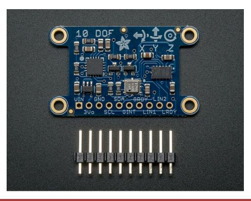
To interface with the sensor, you will need to solder in wire or header into the breakout row at the bottom. You cannot 'press fit' or 'twist' wires in, they will not make good contact! Soldering is required
