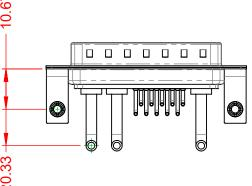
20A (CURRENT) POWER/CO-AX CONTACT RATING: (IF PRESENT) SIGNAL CONTACT CURRENT RATING: 5A PER CONTACT SIGNAL CONTACT RESISTANCE:  $10m\Omega$  MAX. **INSULATOR RESISTANCE:**
