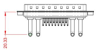
POWER/CO-AX CONTACT RATING:30A (CURRENT)(IF PRESENT)SIGNAL CONTACT CURRENT RATING:5A PER CONTACTSIGNAL CONTACT RESISTANCE: $10m\Omega$  MAX.INSULATOR RESISTANCE:5000MΩ min.DIELECTRICDIELECTRIC
