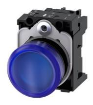
Indicator lights, 22 mm, round, plastic, blue, lens, smooth, with holder, LED module, with integrated LED 230 V AC, screw terminal, with laser labeling, upper case
