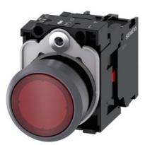
Illuminated pushbutton, 22 mm, round, plastic with metal front ring, red, pushbutton, flat, momentary contact type, with holder, 1NC, LED module with integrated LED 24 V AC/DC, screw terminal, Z=20-unit packaging
